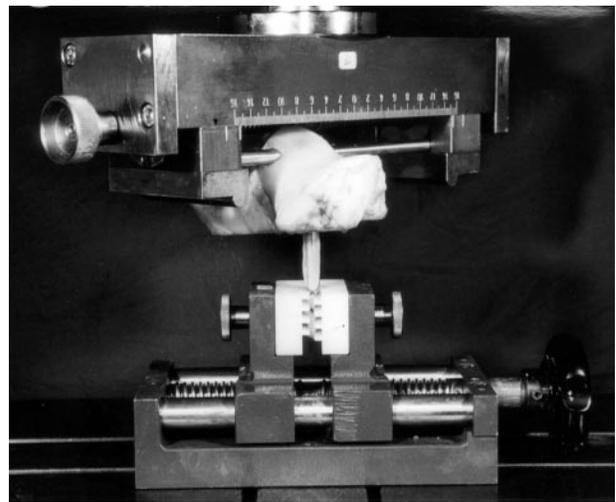
**FIGURE 5.** Construct mounted in material testing machine with the free graft end secured into a custom-made clamping device leaving a 25-mm graft length between the bone surface and the clamp.
