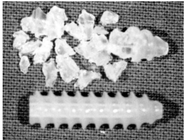
**FIGURE 2.** Bulky fragments of a highly crystalline PLLA interference screw 20 months after implantation compared with a nonused specimen. (Reprinted with permission.<sup>36</sup>)
